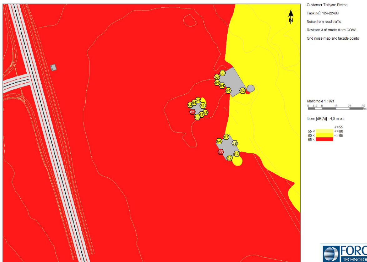
Figure 10 Grid noise map for Revision 3 at 4 m above ground with façade points at 1 st floor.
