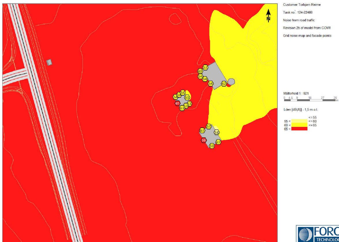
Figure 8 Grid noise map for Revision 2b at 4 m above ground with façade points at 1 st floor.
